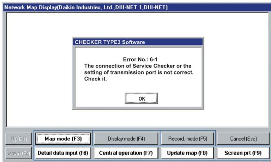
Even though all settings have been made and the window has been switched, if no data is read and the above error is displayed on the window, the following causes will be supposed.
