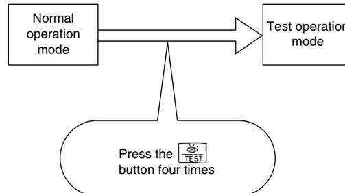
After setting of test operation mode, pressing the
