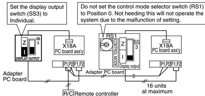
**i Note** The remote controller can be installed on indoor units to which the adapter PC board is not directly connected.
