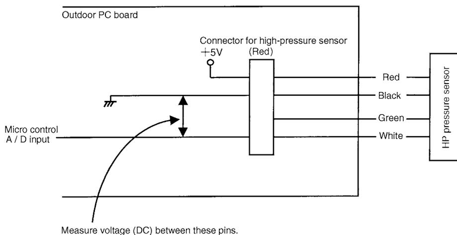
When the color of harness is not as mentioned above, find the measuring point by following procedure.
