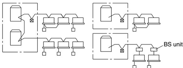
This mode enables a batch of the demand control and the low noise control of outdoor units enclosed with [ \_ \_ ].
