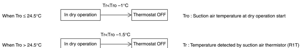
Fan is driven with L flow rate during dry operation, and turned off for a period of 6 minutes during thermostat-off, and then with L flow rate. (In order to prevent humidity from rising in the room during thermostat-off.)
