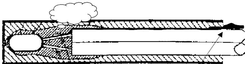
Moisture enters into the thermistor through the clearance between lead wire and filler.
