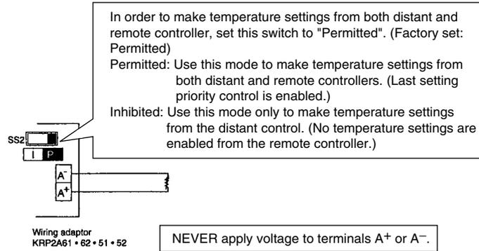
Temperature settings corresponding to resistance values in the range of 0 to 135Ω can be made.
