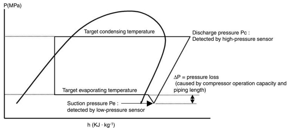
In the compressor capacity controller of VRV system, the pressure detected ( $P_e$  or  $P_c$ ) by pressure sensor installed in outdoor unit is converted into equivalent saturation temperature, and the evaporation temperature ( $T_e$ ) while cooling or the condensation temperature ( $T_c$ ) while heating are so controlled with PI control as to put them close to the target value in order to maintain stable capacity in spite of incessantly varying load. (Refer target value below table.)
