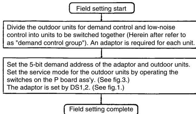
3. To carry out operation mode switching and demand control simultaneously
