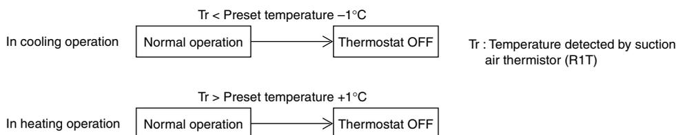
However, the unit can be controlled only by body-thermostat when using 1 group remote controller. For cassette type indoor unit, the unit is controlled with compensation value of  $-2^{\circ}\text{C}$  against body-thermostat detection value in heating operation. (Thermostat - differential can be changed from  $1^{\circ}\text{C}$  to  $0.5^{\circ}\text{C}$  with field setting. Refer to page 43 and page 44 for changing.)
