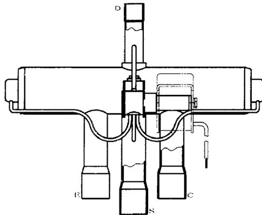
Four way valve is a representative valve which is used for heat pump type air conditioner. This valve functions to selection flow direction of superheated refrigerant discharged from compressor. In heating operation, the valve feeds the refrigerant to indoor heat exchanger. While in cooling and defrosting in heating, the valve feeds to outdoor heat exchanger.
