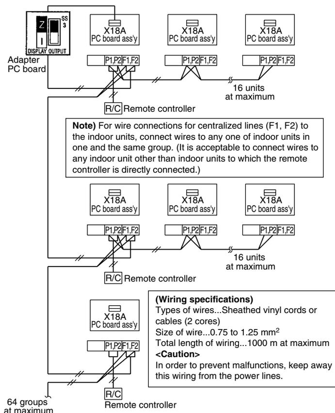
**Wiring to External Controller (e.g. Centralized Control Monitor)**
