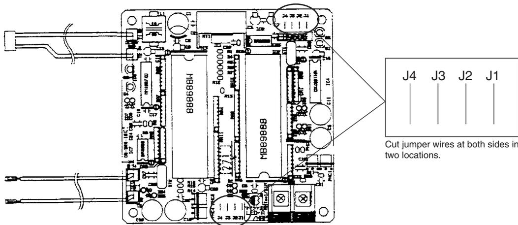
Cut the jumper wire “J2”. → The use of expander adapter in combination with thermal storage controller will be enabled.
