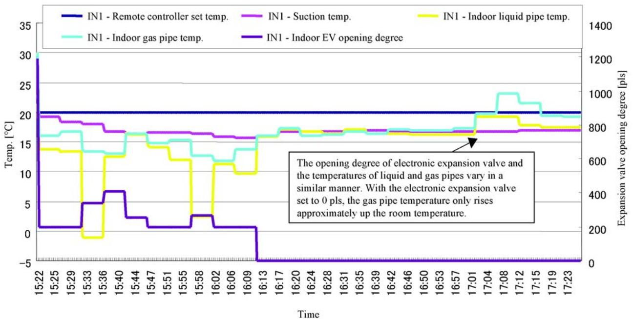
**(Case Example) Ve-up STD RSXYP 5-10L:Malfunction of heating (Indoor units are all in fan operation mode.)**
