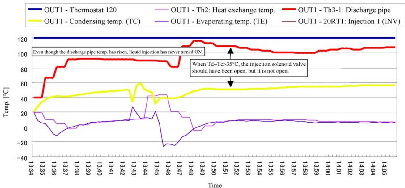
**(Case Example) VRV II Heat recovery type: Malfunction of heating**
