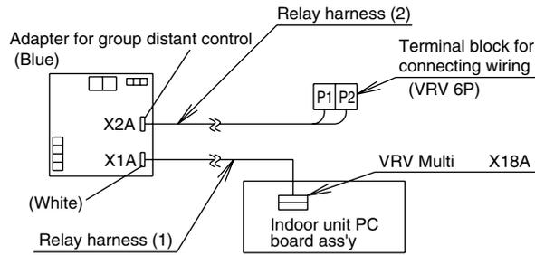
Use the relay harnesses (1) and (2) provided to connect wires as shown in figure above.
