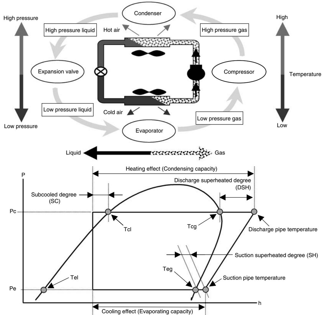
Theoretic refrigeration cycle neglecting pressure loss, etc. drawn on P-H diagram is shown as above.
