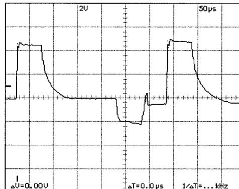
Above abnormal waveforms are generated due to field factors. Some countermeasures shown in below table can be applied at the equipment side, and conduct proper measure according to the state of waveform.
