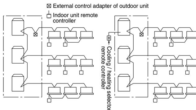
This mode enables a batch selection of operation mode of outdoor units enclosed with [ \_ \_ ].
