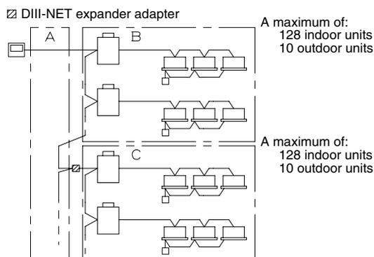
In the ranges of B and C, a maximum of 128 indoor units and 10 outdoor units are connectable, respectively.
