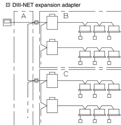
In the ranges of A, B, and C, wirings of 1000-m maximum distance, 2000-m total wiring length, and 16 maximum branches are enabled, respectively.
