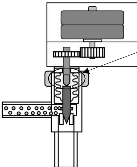
The valve is protruded excessively into the valve seat.
