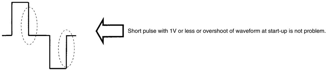
When the waveform as shown below appears in measuring of transmission waveform, transmission malfunction may probably be caused.
