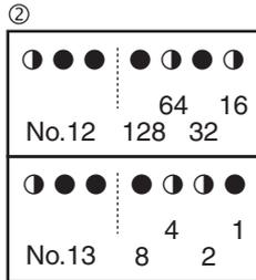
For example, the number of terminal units for Nos. 12 and 13 is expressed in eight-digit binary number, which are the combination of four upper and four lower digits for Nos. 12 and 13 respectively. (0 to 128)
